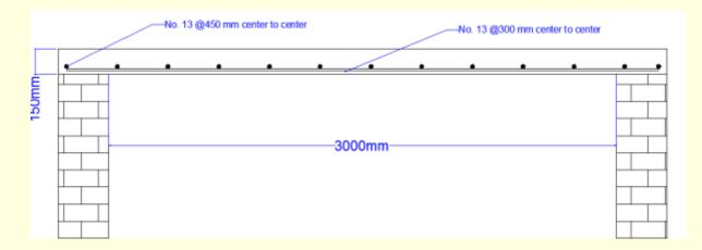
**Example 3:-** Design the one-way slab shown in the accompanying figure to support a live load of 12 kN/m<sup>2</sup>. Do not use the ACI thickness limitation for deflections. Use  $\rho = \rho_m$ , =28MPa and  $f_y$ =420MPa
