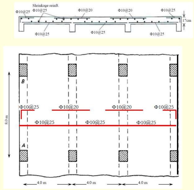
**Example 2**:- A one-way single-span reinforced concrete slab has a simple span of 3m and carries a live load of 5.75 kN/m<sup>2</sup> and a dead load of 0.96 kN/m<sup>2</sup> in addition to its self-weight. Design the slab and the size and spacing of the reinforcement at mid-span assuming a simply supported moment, given:  $f_c = 28MPa$  and  $f_y = 420MPa$
