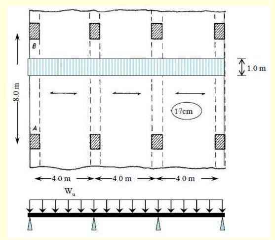
**3- Calculate the factored load wu per unit length of the selected strip:** Own weight of slab =  $0.17 \times 25 = 4.25 \text{ kN/m}^2$  $W_u = 1.20 (3+4.25) +1.60 (3) = 13.5 \text{ kN/m}^2$ For a strip 1 m wide,  $W_u = 13.5 \text{ kN/m}$
