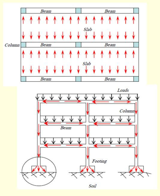
Slabs are flexural members. Their flexure strength requirement maybe expressed by: $Mu \leq \Phi Mn$ 7.5.1.1ACI code318M-14
