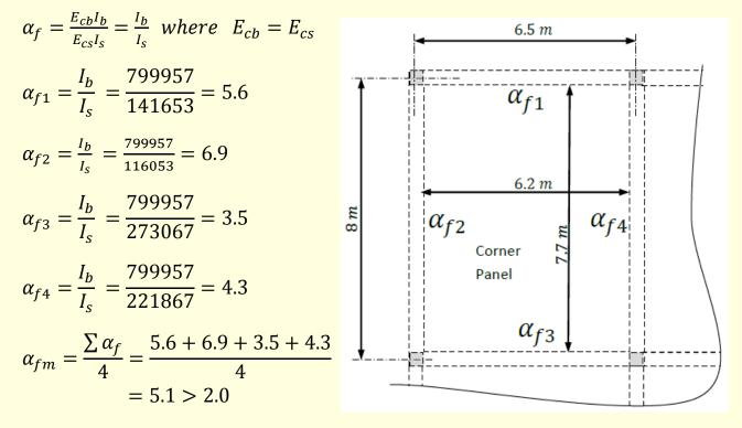
$\alpha_{fm} = 5.1 > 2.0$  the minimum slab thickness will be:
